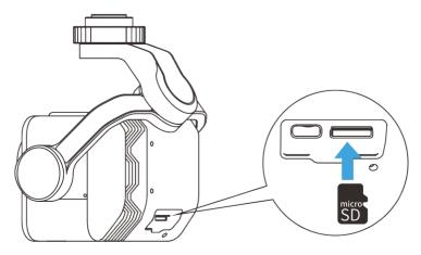
Fig 3-18 Installing the microSD Card
