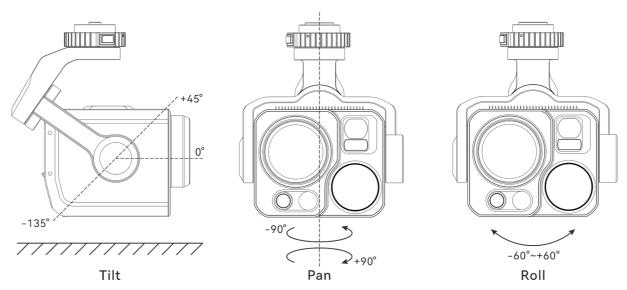
Fig 3-14 Mechanical Rotation Range of DG-L35T Gimbal
