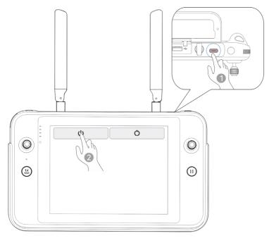
Fig 4-7 Turning the Remote Controller Off
