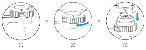
Fig 3-16 Removing the Gimbal
