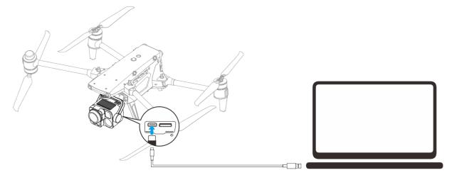
Fig 3-19 Connect to PC/MAC via Gimbal USB-C Interface
