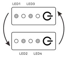
Fig 5-5 Self-heating State
