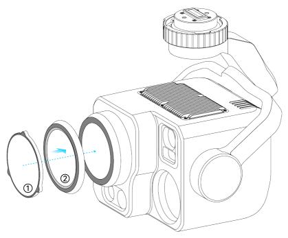
Fig 3-17 Installing ND filter
