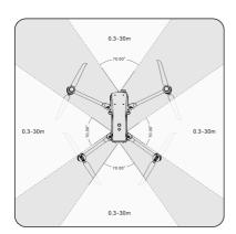
Fig 2-4 Observation Range of Millimeter-wave Radars
