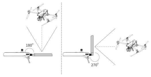
Fig 4-10 Extend the antenna
