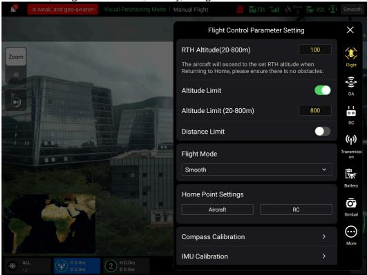
Fig 6-4 "Flight Control Parameter Setting" interface
