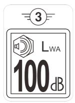
Fig 3-20 A-weighted sound power level of the Autel Alpha multi-rotor drone
