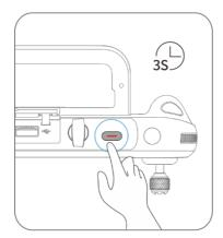
Fig 4-6 Turning the Remote Controller On
