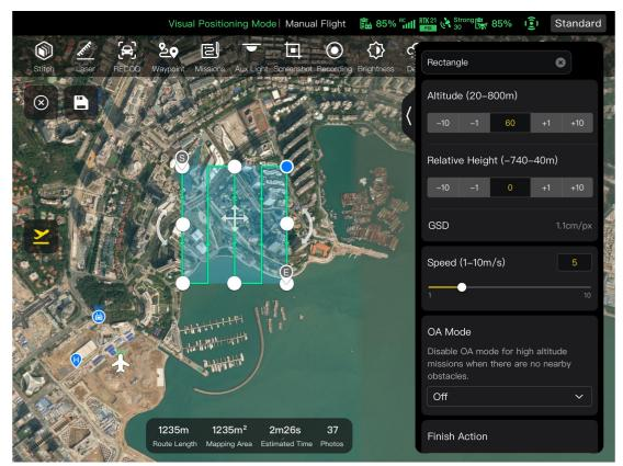
Fig 6-9 Rectangle Mission Interface (Before taking off)
