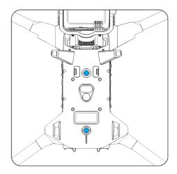
Fig 2-3 Upper left, upper right, and bottom visual lens modules of the aircraft
