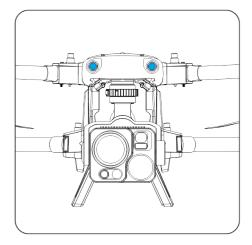
Fig 2-2 Front and rear visual lens modules of the aircraft
