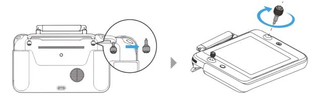
Fig 4-5 Installing command sticks
