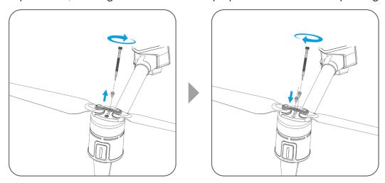
Fig 3-8 Install the Propellers
