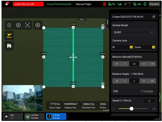
Fig 6-10 Polygon Mission Interface (Before taking off)
