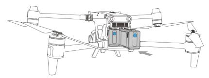
Fig 5-2 Install the Smart Battery
