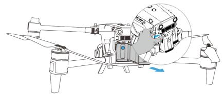
Fig 5-3 Remove the Smart Battery
