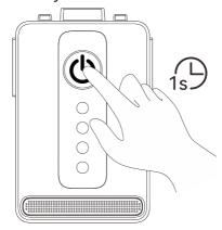
Fig 5-4 Checking Battery Level
